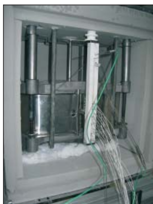
2 kW stack integrated in a demonstration system
